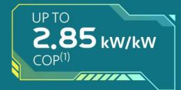
(1) Nominal Capacity, COP, and IPLV based on AHRI 551/591 conditions @ 12°C/ 7°C EEWT/ELWT, 35°C Ambient Temperature
